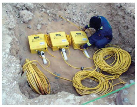
A proper PMM installation will help monitor fracture growth, increase production and avoid induced seismicity events that have the potential to put lives at risk and cause substantial damage to equipment and nearby structures.
